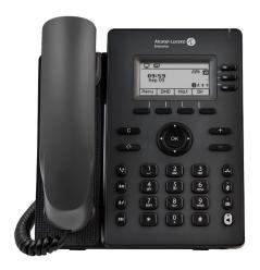
The ALE-2 is configured with a 2.8-inch backlit, black-and-white display that can accommodate up to four lines of texts and support up to 1000 contacts and call logs. The five-way conferencing, local directory, and three separate lines make it easy for all departments to communicate. This phone is compliant with the interoperable SIP standard and offers secure communications for remote workers using a SIP Session Border Controller.
